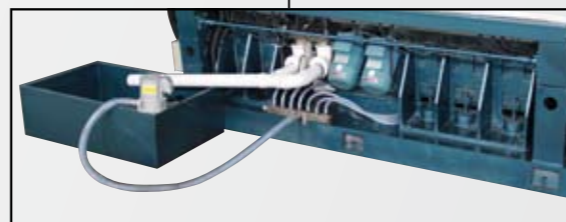
PVC快速排水与不锈钢进水系统 PVC rapid drainage and stainless steel water intake system
